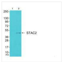
Western blot analysis of extracts from cos-7 cells (Lane 2), using STAC2 antiobdy. The lane on the left is treated with synthesized peptide.
