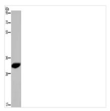
Gel: 8%SDS-PAGE, Lysate: 40 µg, Lane: 231 cells, Primary antibody: CSB-PA921993(HMGN5 Antibody) at dilution 1/100, Secondary antibody: Goat anti rabbit IgG at 1/8000 dilution, Exposure time: 5 minutes
