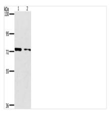
Gel: 6%SDS-PAGE, Lysate: 40 µg, Lane 1-2: MCF7 cells, hela cells, Primary antibody: CSB-PA296760(PPP1R13L Antibody) at dilution 1/500, Secondary antibody: Goat anti rabbit IgG at 1/8000 dilution, Exposure time: 30 seconds
