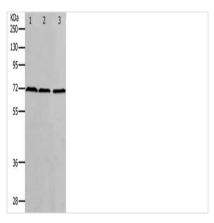
Gel: 10%SDS-PAGE, Lysate: 40  $\mu$ g, Lane 1-3: K562 cells, hela cells, 293T cells, Primary antibody: CSB-PA077190(PRMT5 Antibody) at dilution 1/400, Secondary antibody: Goat anti rabbit IgG at 1/8000 dilution, Exposure time: 2 minutes
