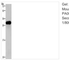
Gel: 10%SDS-PAGE, Lysate: 40 µg, Lane: Mouse stomach tissue, Primary antibody: CSB-PA058956(PSCA Antibody) at dilution 1/200, Secondary antibody: Goat anti rabbit IgG at 1/8000 dilution, Exposure time: 5 minutes
