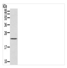
Gel: 12%SDS-PAGE, Lysate: 40 µg, Lane: Human placenta tissue, Primary antibody: CSB-PA239746(IL31 Antibody) at dilution 1/200, Secondary antibody: Goat anti rabbit IgG at 1/8000 dilution, Exposure time: 1 minute
