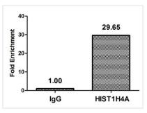
Chromatin Immunoprecipitation Hela (4\*10<sup>6</sup>, treated with 10mM sodium propionate for 4h) were treated with Micrococcal Nuclease, sonicated, and immunoprecipitated with 5µg anti-HIST1H4A (CSB-PA010429OA16propHU) or a control normal rabbit IgG. The resulting ChIP DNA was quantified using real-time PCR with primers against the  $\beta$ -Globin promoter.
