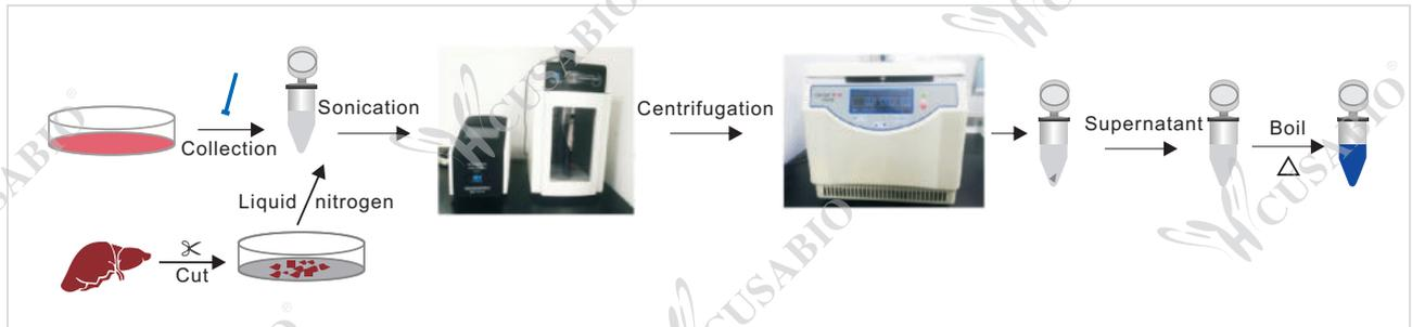
Fig. 2. The processes of lysate preparation
